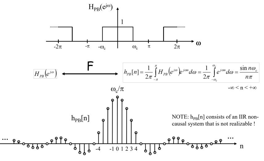
NOTE+: the response  $h_{PB}[n]$  is not absolutely summable, but its square is summable, which highlights the fact that a filter resulting fom  $h_{PB}[n]$  by limiting its length, is the best approximation, in the mean-square sense, to  $H_{PB}(e^{j\omega})$  (*i.e.* to the ideal filter).
