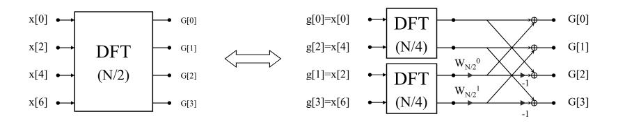
$\rightarrow$  its computational cost (multiplications) is proportional to  $2(N/4)^2+N/4=N^2/8+N/4$ , making that if this structure is used in the computation of G[k] and H[k], the total computational cost (multiplications) involved in the computation of X[k] is proportional to  $2\times N^2/8+2N/4+N/2=N^2/4+N$ .
