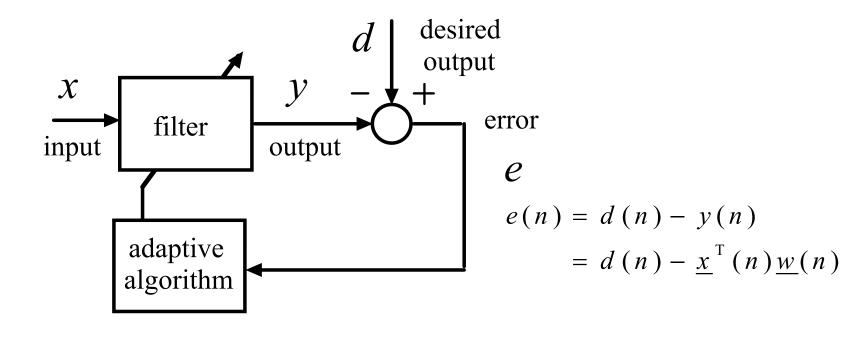
$$e^{2}(n) = d^{2}(n) - 2d(n)\underline{x}^{T}(n)\underline{w}(n) + \underline{w}^{T}(n)\underline{x}(n)\underline{x}^{T}(n)\underline{w}(n)$$
