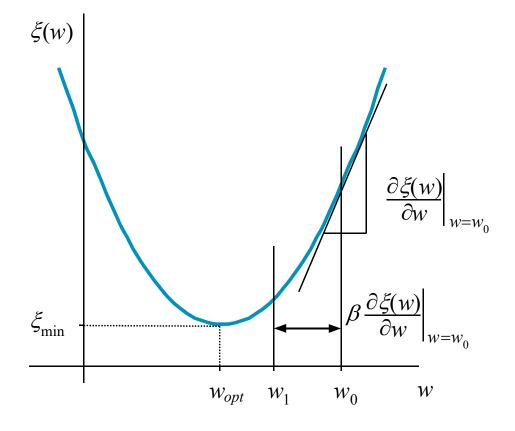
$$\frac{\partial \xi(\underline{w})}{\partial \underline{w}} = \frac{\partial}{\partial \underline{w}} \left( E\left[d^{2}(n)\right] + \underline{w}^{\mathrm{T}}R \underline{w} - 2\underline{p}^{\mathrm{T}}\underline{w} \right)$$
